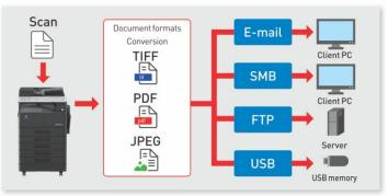
The scanned files can be saved directly to USB memory, or sent to different destination such as E-mail, SMB or FTP. The supported scan formats are TIFF, PDF and JPEG.
