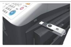
Connect USB memory to print data directly or save scanned data to the USB memory
